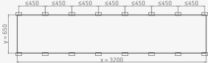
H2. Max. Design wind load: 1,5 kN/m²
