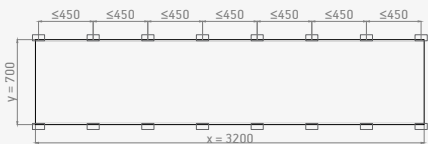
H1. Max. Design wind load: 1 kN/m²
